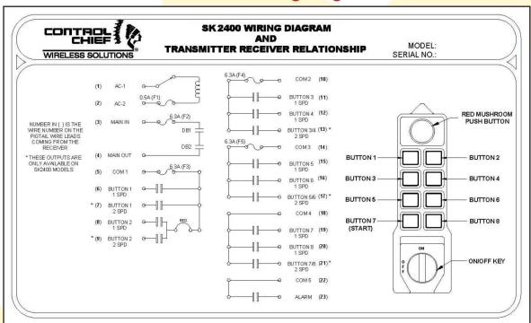
Wiring diagrams for reference only - not for installation
